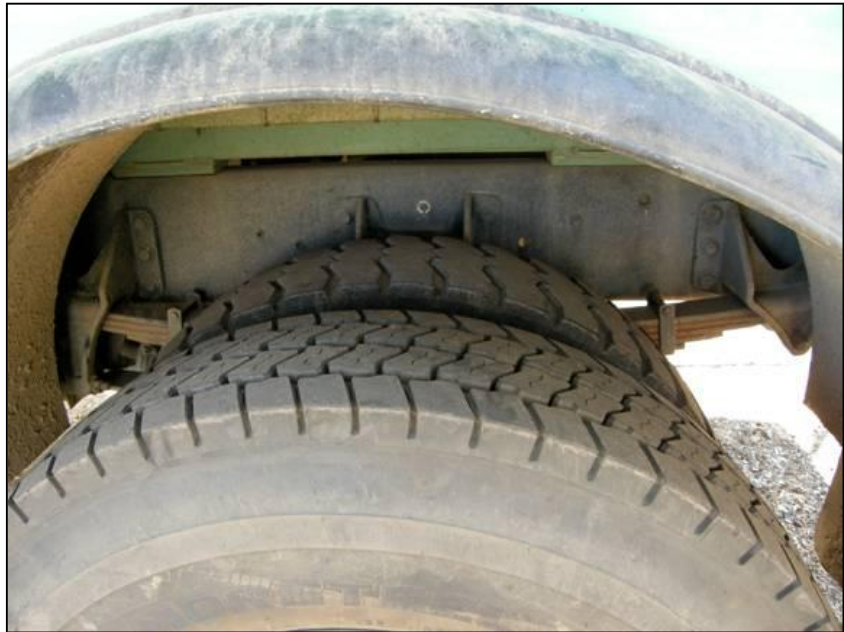
Fig 2 – The replaced outside rear dual on Engine 56. Findings revealed a difference greater than one-inch diameter between the two tires.
